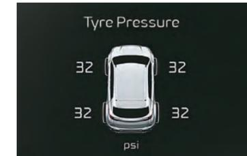
Displays real-time tyre pressure information and alerts if the pressure falls below the recommended levels
