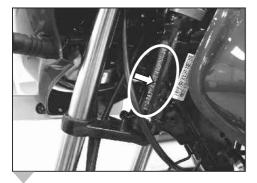
Frame Number Location On Side of Steering Tube (Alpha-Numeric - 17 Digits) Engine Number Location On LH Side Crankcase Near Gear Change Lever (Alpha-Numeric - 11 Digits)
