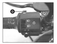
To stop flashing, press the switch IN.
