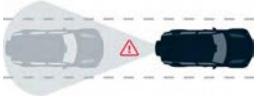
**Rear Pre-collision Monitor** - If a vehicle approaching from behind is not slowing down, Defender will attempt to alert the approaching driver to brake by automatically flashing the hazard lights.
