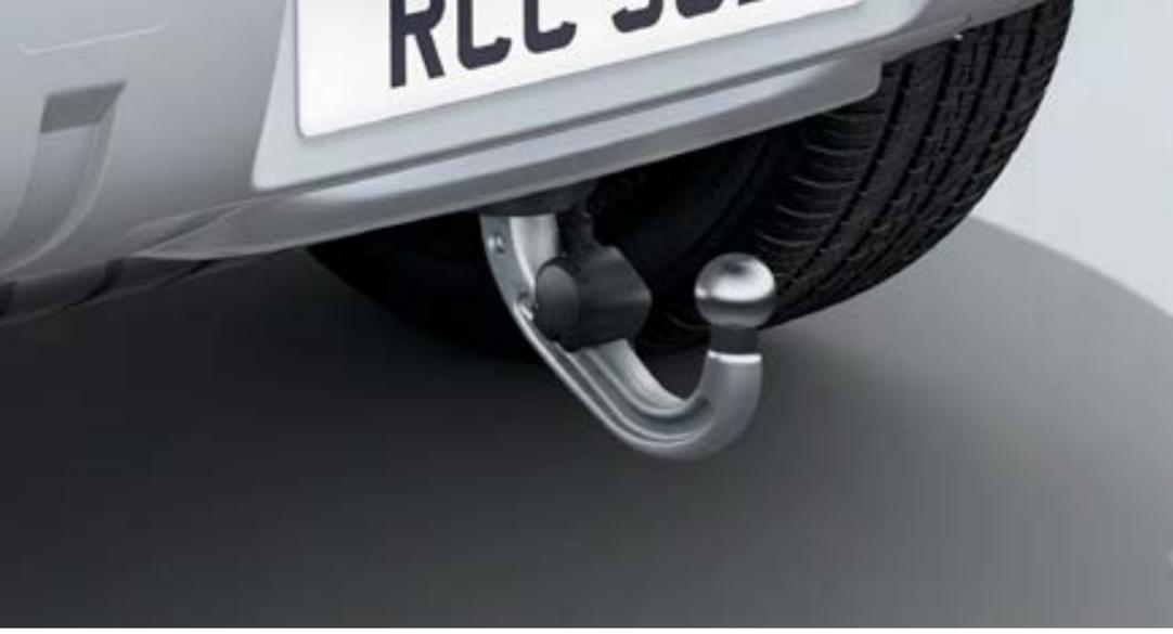
**Electrically Deployable Tow Bar** - Stowed discreetly behind the rear bumper, providing a clean finish. It is designed to deploy/stow in 12 s and is operated via a switch in the rear loadspace, or by the infotainment system in the cabin.
