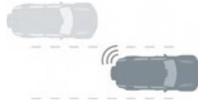
**Blind Spot Assist** - Can help prevent collisions. If your Defender detects another car in your blind spot when you begin to change lanes, a rotational force is automatically applied to the steering wheel - indicating a steering correction should be made.
