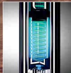
*When big bumps are encountered, the hydraulic cushions keep suspension movement controlled and progressive.*
