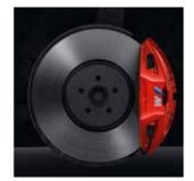
The powerful M Sport brake featuring four-piston fixed calipers at the front and single-piston floating calipers at the rear in Red high-gloss with M logo and featuring large brake discs to ensure an outstanding braking power. Adapted to the vehicle's dynamic potential, it guarantees exceptional braking even with a sporty driving style.
