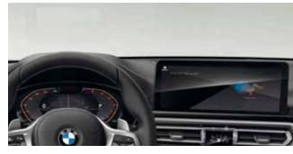
The BMW Live Cockpit Professional with navigation function includes two high-quality displays consisting of a high-resolution 12.3" Control Display that can be operated by touch and a fully digital 12.3" instrument display. The BMW Operating System 7 can also be operated via the iDrive Touch Controller.
