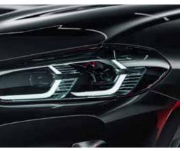
The standard Adaptive LED headlights include low-beam and no-dazzle high-beam headlights (BMW Selective Beam) and turn indicators with full LED technology. The equipment also features cornering lights, daytime running lights and Adaptive headlights with variable light control for excellent illumination of the road ahead and
