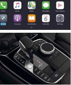
The 8-speed Steptronic Sport transmission offers incredibly sporty gear changes. Whether automatic or manual using the selector lever or gearshift paddles – for comfortable coasting or incredibly dynamic driving. In SPORT mode and with the selector lever in the left-hand S/M position, the gear shifts are configured for the maximum performance.
