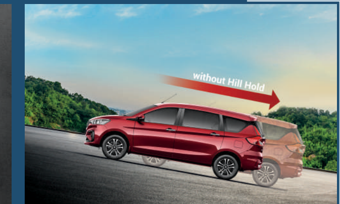
Hill Hold Technology Prevents the car from rolling back momentarily.
