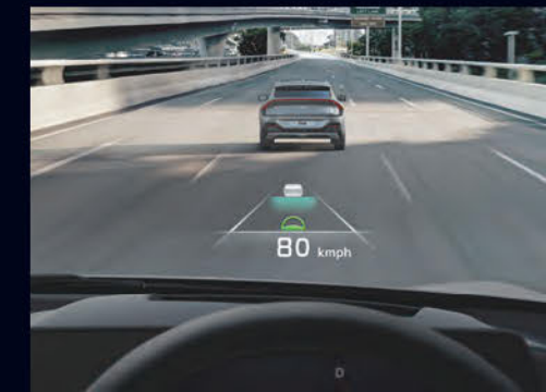
Augmented Reality Head-up Display Key information such as speed, lane safety indication, is projected in an intuitive manner on the windscreen
