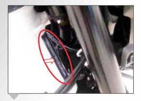
**Frame Number Location** On RH Side of Steering Tube (Alpha-Numeric - 17 Digits) **Engine Number Location** On LH Side Crankcase Near Gear Change Lever (Alpha-Numeric - 11 Digits)
