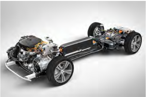
The V60 has been designed from the ground up with plug-in hybrid power in mind, so the batteries and electric motor are set lower in the chassis. This means more responsive, intuitive handling due to a lower center of gravity and more even weight distribution.
