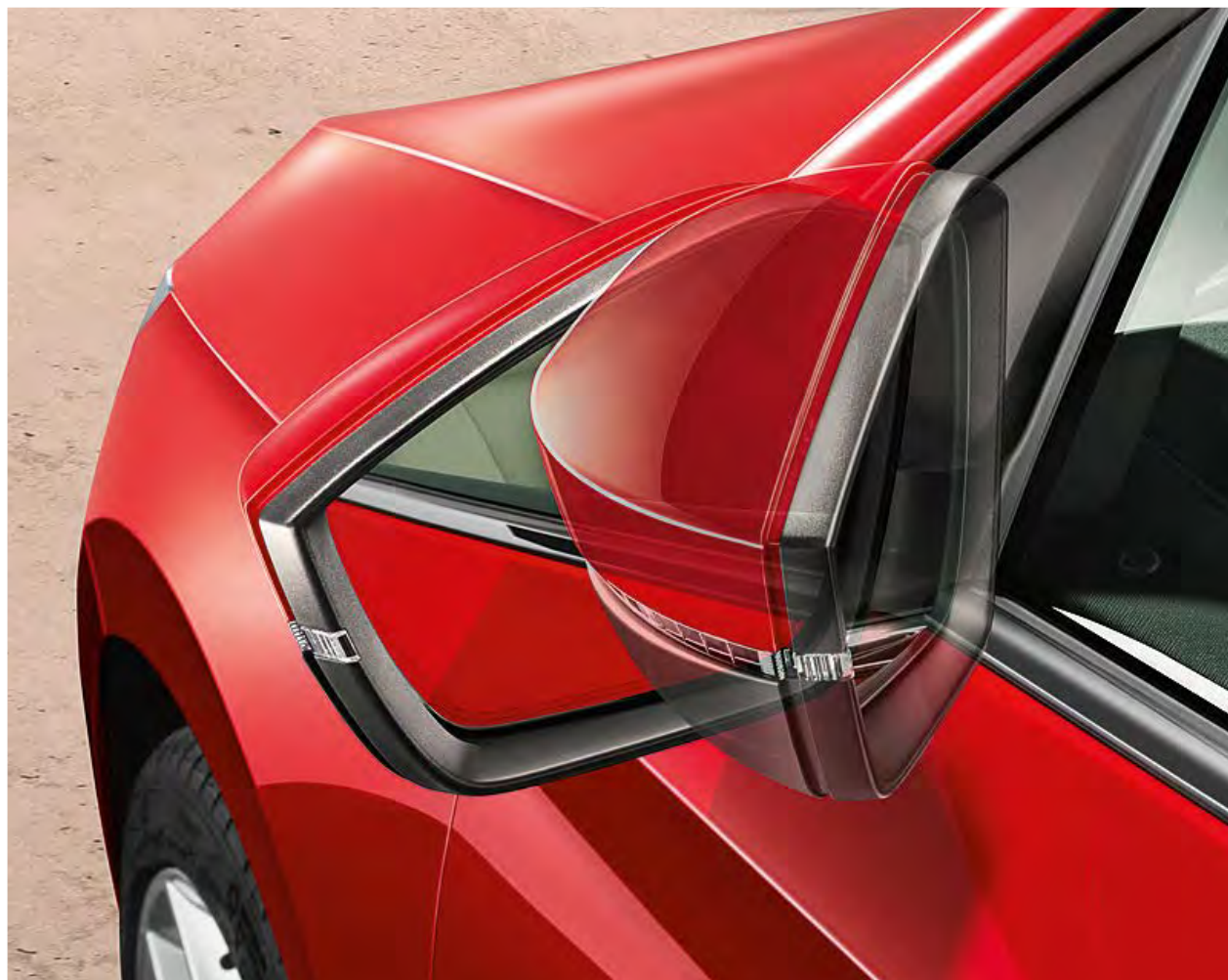
ELECTRICALLY ADJUSTABLE AND HEATED DOOR MIRRORS
