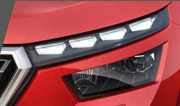
FULL LED HEADLIGHTS With adaptive front light system, dynamic indicators, cornering function and fog lights.
